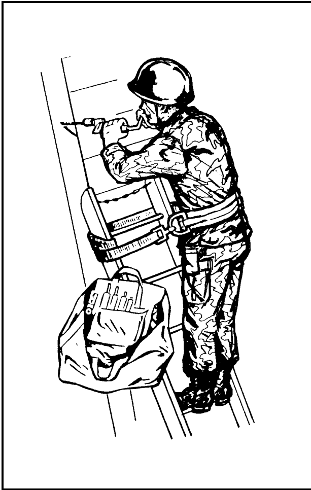
Figure 13-2. Proper use of a safety strap while working from a ladder
